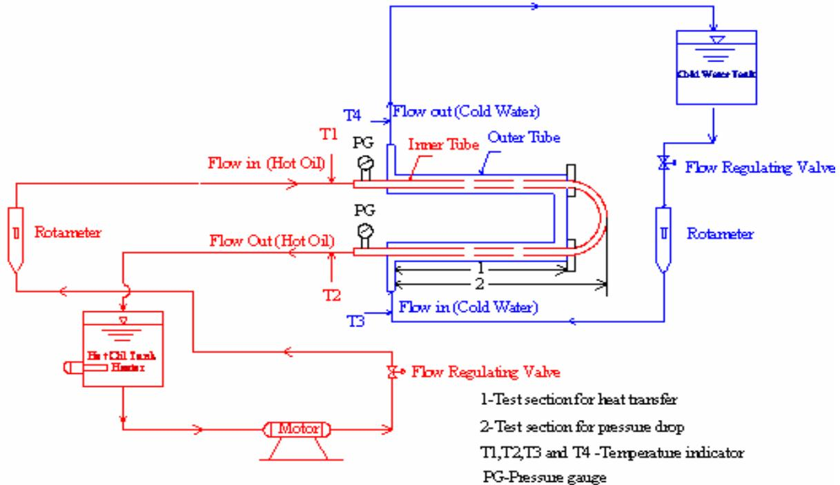
Figure 1: Schematic Diagrams of Experimental Setup.
