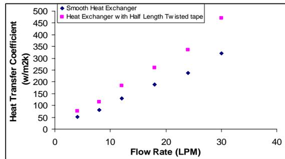
Figure 3: Flow rate vs. heat transfer coefficient.
