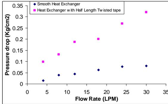
Figure 4: Pressure drop ( $\Delta P$ ) Vs. Flow rate.
