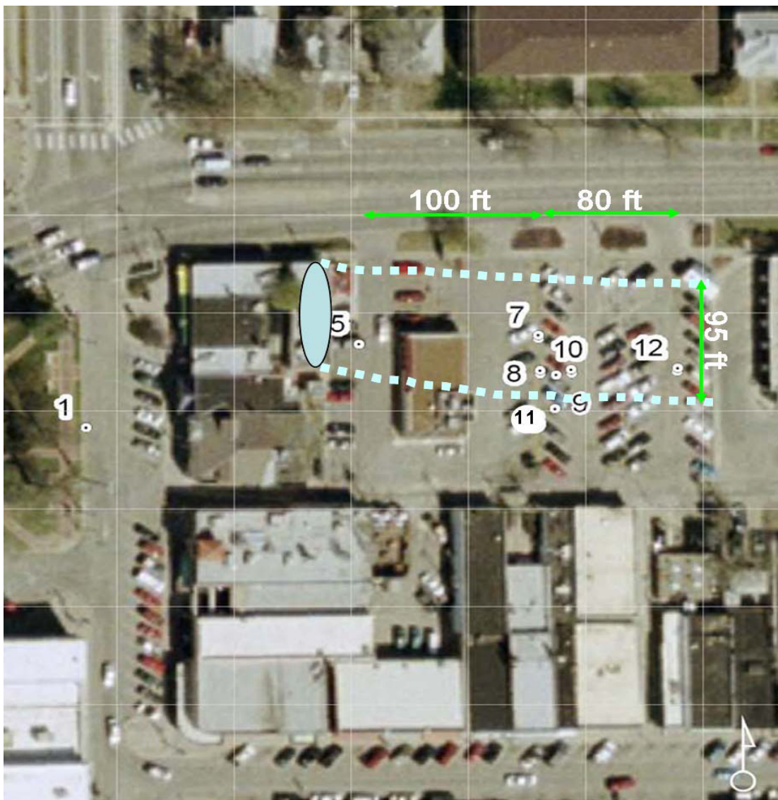
Figure 2. GIS aerial map showing location of PCE source (Oval shape), direction and width of contaminating plume (Dashed lines) in the pilot study area.
