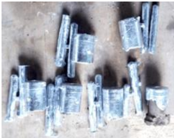
Figure 9. Unmachined cast pistons
