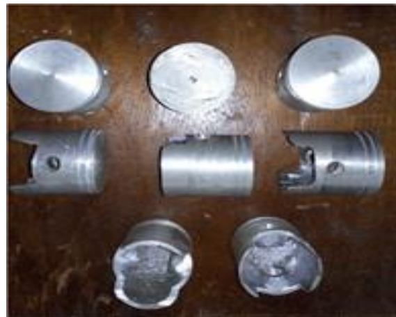
Figure 10. Machined cast pistons
