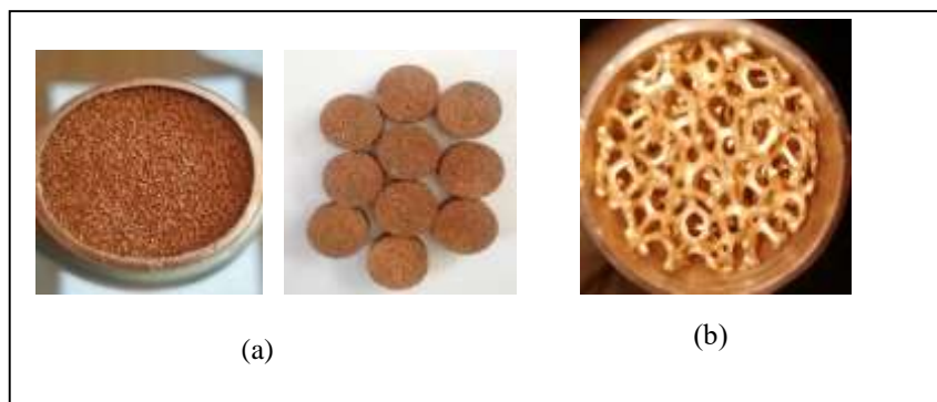
Figure 4. Photograph of test section and type of metal foam inside the pipe (a) 40 PPI (b) 10 PPI
