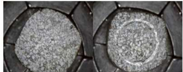
(vi) Developed brake pad sample with 500µm particle size
