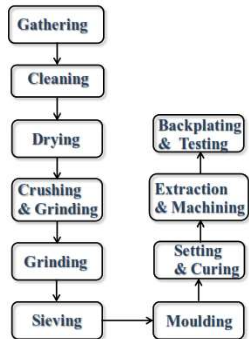
Figure 1. Flowchart of brake pad development process (Ossia et al. [21])
