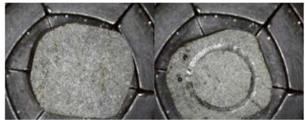
(iv) Developed brake pad sample with 125µm particle size
