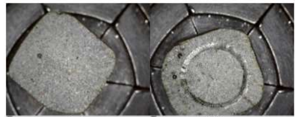
(v) Developed brake pad sample with 250µm particle size
