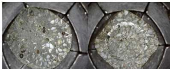
(vii) Developed brake pad sample with 850µm particle size
