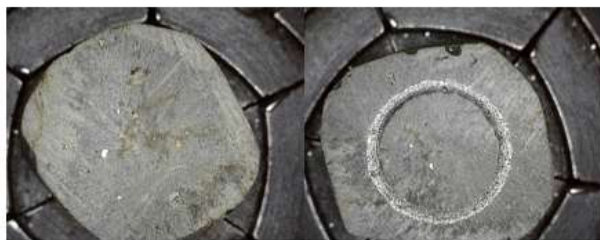
(ii) Developed brake pad sample with 63µm particle size
