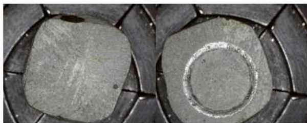
(iii) Developed brake pad sample with 90µm particle size
