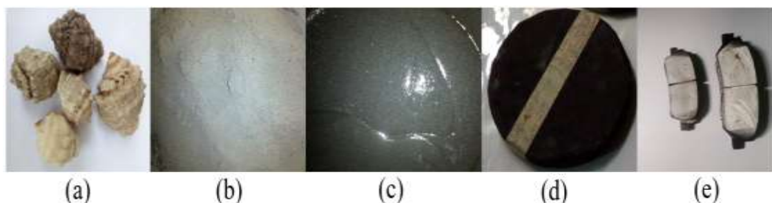
Figure 2. Brakepad development process: (a) uncrushed Thais Coronata shells, (b) crushed Thais Coronata shells, (c) homogenous mixture, (d) heat-treated sample, (e) machined finished product
