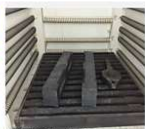
Mold inside the furnace
