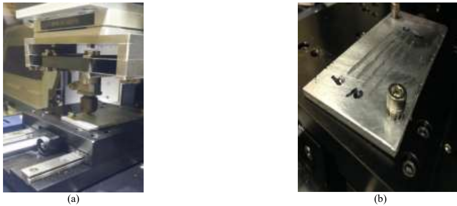
Figure 3. (a) pin-on-disc machine used for wear test, (b) The sample that is subjected to wear testing.
