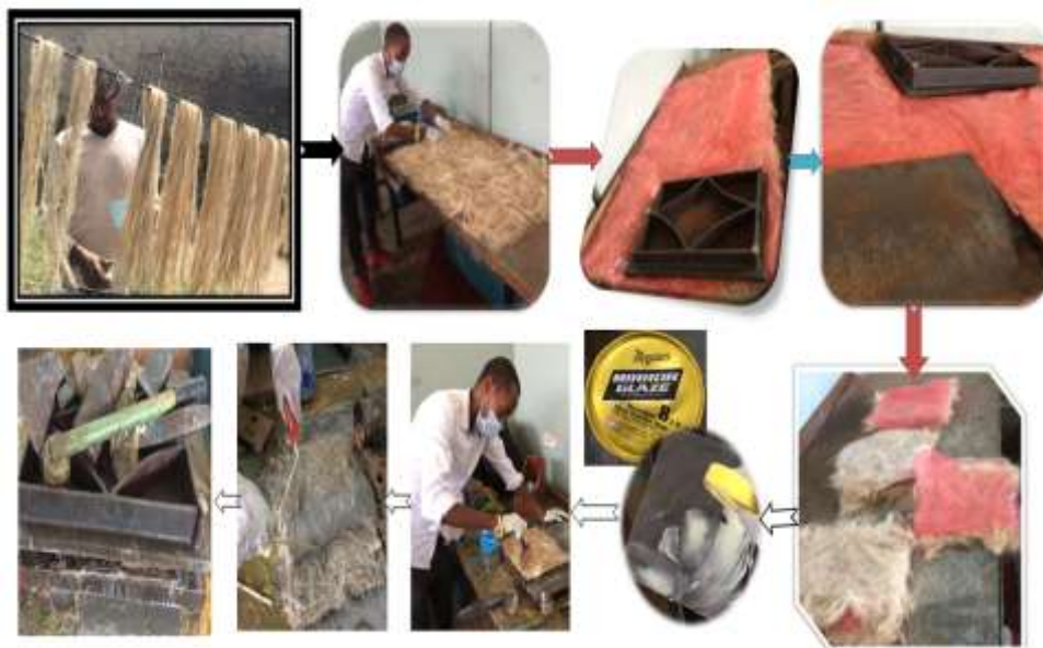
Figure 2. Banana fibre reinforced polymer composite fabrication procedures
