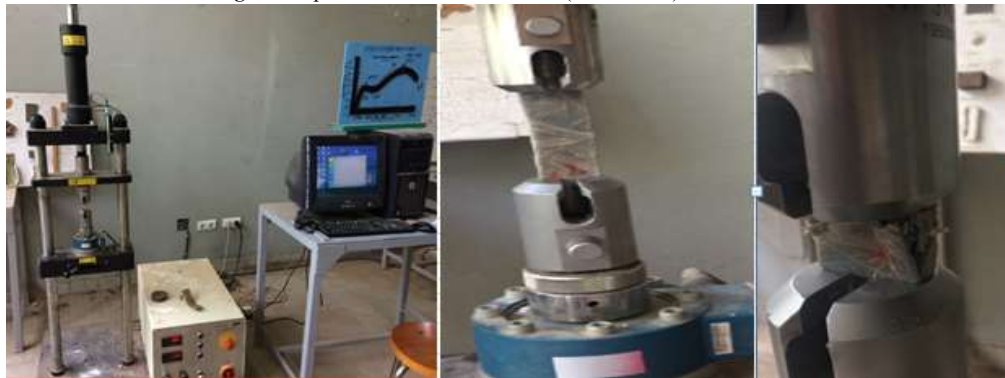
Figure 6. Compression Stress testing UTM-50kN
