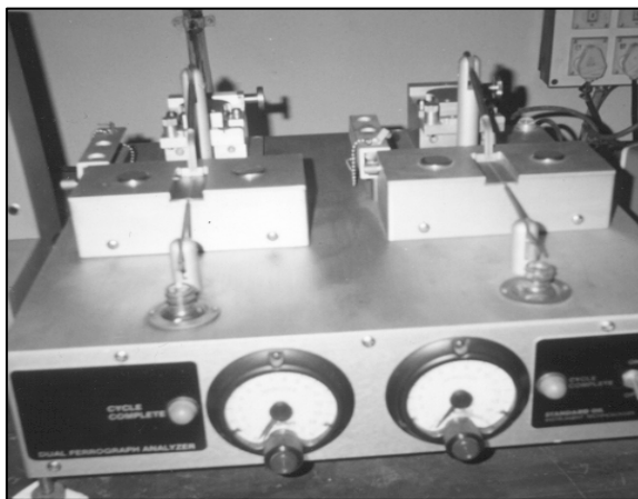
Figure 6 : Dual ferroanalyzer for ferrogram preparation.
