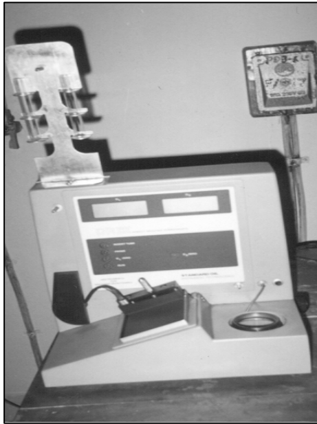
Figure 4: DRIII system for wear separation.
