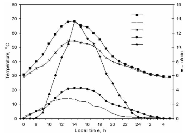
Figure 6. Variation in temperatures and production rate for laboratory still with varying input – set II.
