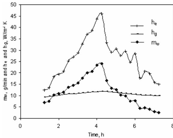
Figure 8. The variation in heat transfer coefficient and production rate for laboratory still with 1500 W constant input.
