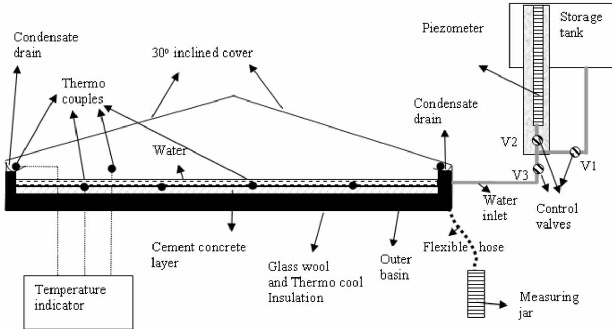
Figure 2. Single basin double slope solar still.
