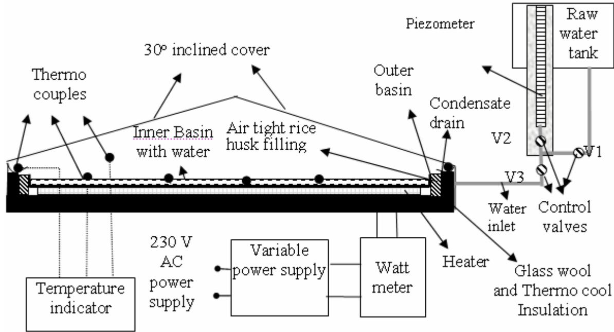
Figure 1. Single basin double slope laboratory still.
