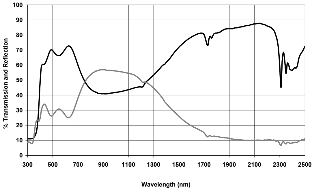
Figure 1. Spectral transmission and reflection of Solarflair 870 pigment particles
