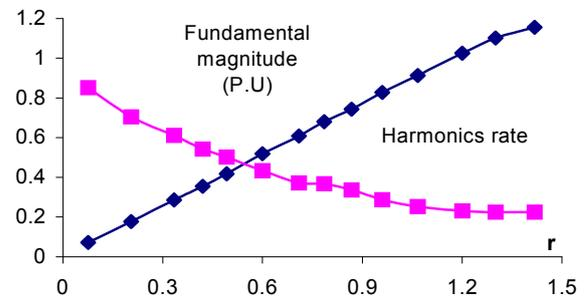
Figure 6 The adjusting characteristic of the output voltage of the inverter
