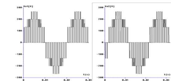
Figure 12. Output voltage of two three level inverter
