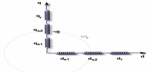
Figure 2. Representation of DSIM in the Park frame
