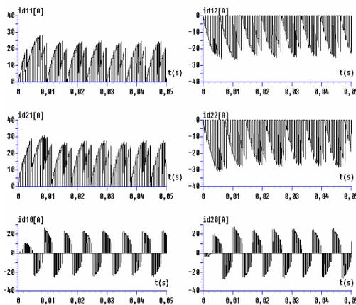
Figure 11. Input currents of the two three-level inverter
