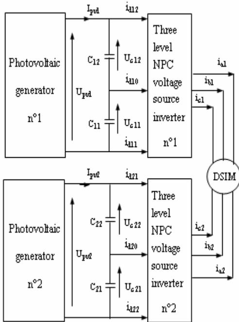
Figure 7. Two photovoltaic generator-filter-two three-level NPC VSI-DSIM cascade
