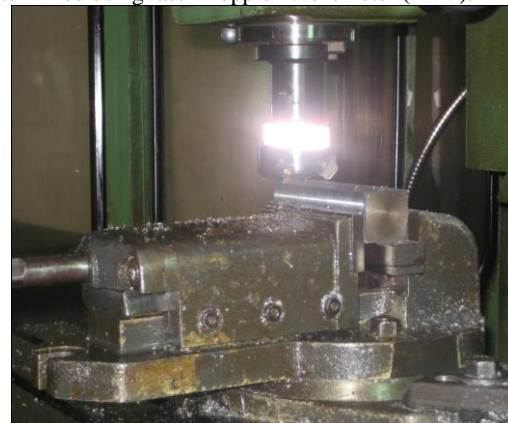
Figure 3: Face milling teeth are spaced around the circumference of the cutter body.
