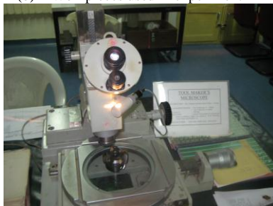
(c) Tool maker's microscope for flank wear.
