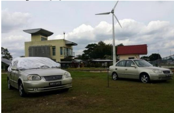
Figure 5. Two identical cars parked in the sun, with/ without a solar reflecting cover.[74].
