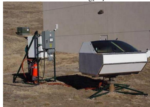
Figure 8. Passenger compartment mockup for heat-pipe IP cooling testing [61].
