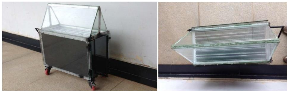
Figure 25. Experimental device of extraction water in the arid region using Silica Gel[136].
