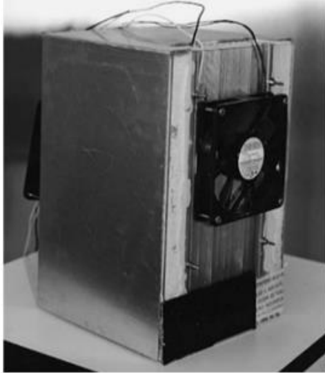
Figure 36. Prototype thermoelectric dehumidifier for water production[167].
