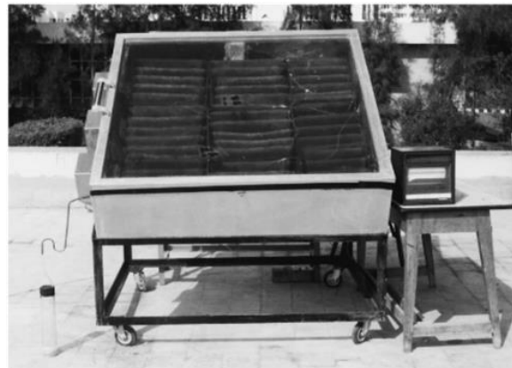
Figure 12. Image of desiccant and a solar collector used for AWG [106].
