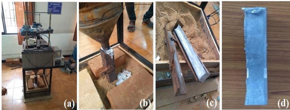
Figure 6. (a) Stir Casting Setup, (b) Poured Specimen, (c) Allowed to Cool, (d) Final Specimen
