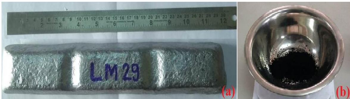
Figure 5. (a) As-Cast Ingot of LM29 Alloy and (b) As-received Multi Walled Carbon Nanotubes
