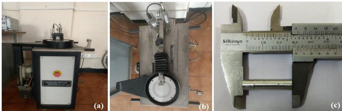
Figure 7. (a) Front View and (b) Top view of the Pin on Disc Setup and (c) Specimen for Pin on Disc experiment
