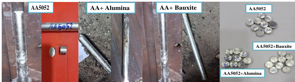
Figure 3. Samples prepared by stir casting
