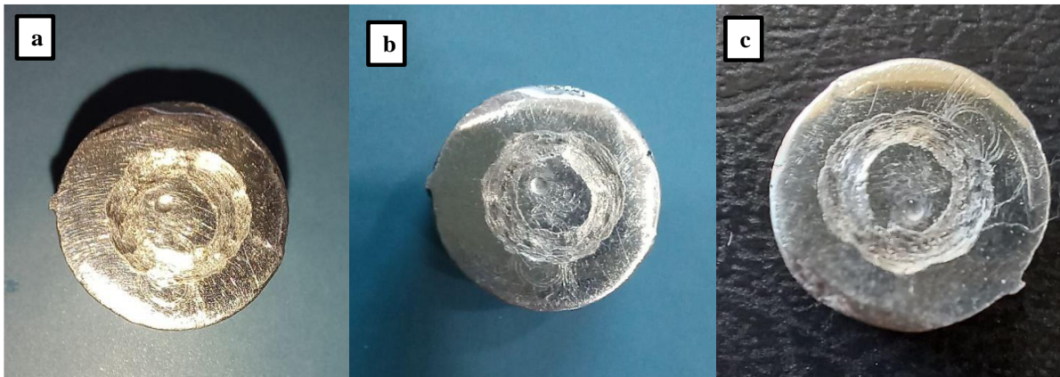
Figure 16. Effect of wear test relative to: (a) AA5052, (b) AA5052 reinforced with alumina and (c) AA5052 reinforced with bauxite.
